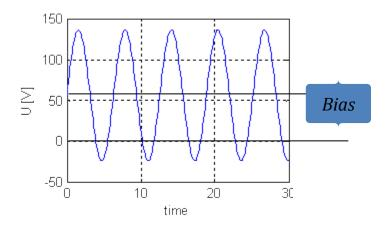
Since most RF amplifiers are AC coupled, they will strip any DC component off the signal applied. Therefore, this needs to be added to the amplified signal to be applied to the load (crystal).
