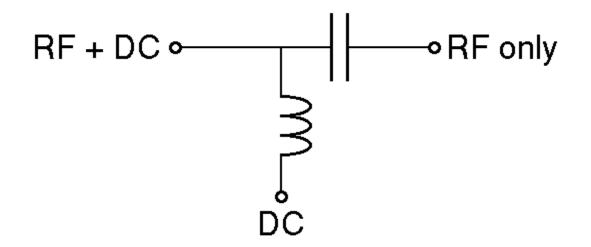
The output of the amplifier will be connected to the port designated **RF only** and the DC voltage is applied to the port designated **DC**. The capacitor will allow the RF to pass through with little loss while preventing the DC from feeding back to the amplifier. The inductor allows the DC to pass without loss while providing high impedance to the RF. Basically, this allows us to combine the two signals and apply both the RF signal and DC bias to our load.
